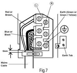
If the supplied plug is cut off dispose of it safely as it will be a shock hazard if inserted into a 13 amp socket elsewhere in the house.
